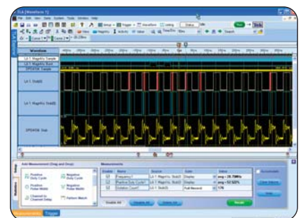
► Tektronix' Integrated View feature (iView™) fully integrates the performance and measurement accuracy of a Tektronix oscilloscope with the multi-channel and powerful triggering capabilities of a Tektronix logic analyzer in one display, allowing designers to quickly verify and debug their designs.
